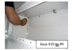
Bolt 3<sup>rd</sup> Compartment Bench to 3<sup>rd</sup> Compartment Divider using ½" x ¾" carriage bolts and serrated nuts. Nuts should be on the inside of the bench
